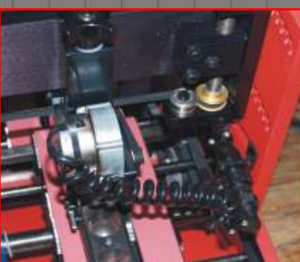
Dynamic Rotation Technology separators that can be removed and slide to the position needed.
