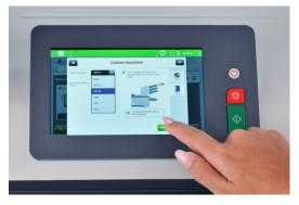
The intuitive, full-colour, high resolution 7" touch-screen provides a wizard-based user-friendly interface, making it easy for anyone to select and run their folding and inserting jobs.
